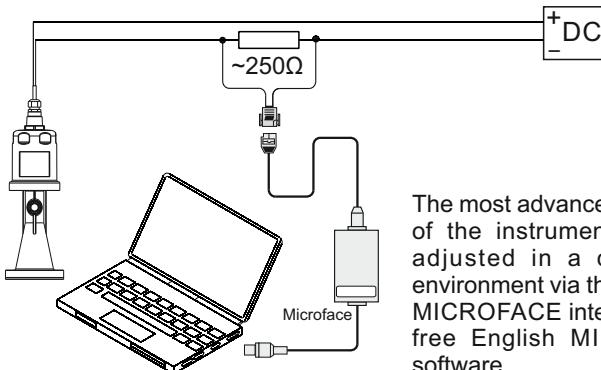
The most advanced settings of the instrument can be adjusted in a computer environment via the optional MICROFACE interface with free English MICROWIN software.
