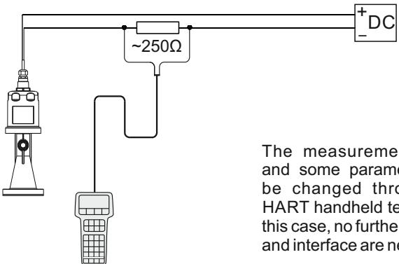
The measurement range and some parameters can be changed through the HART handheld terminal. In this case, no further software and interface are needed.
