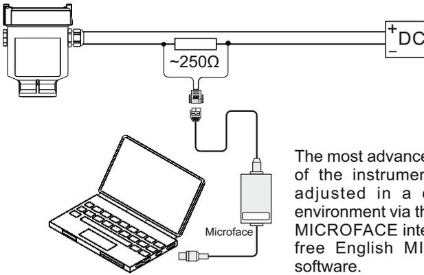
The most advanced settings of the instrument can be adjusted in a computer environment via the optional MICROFACE interface with free English MICROWIN software.
